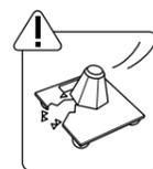
The weighing surface is made of glass. Do not let hard or heavy objects fall onto it. There is a danger that the glass could shatter and cause injury.
